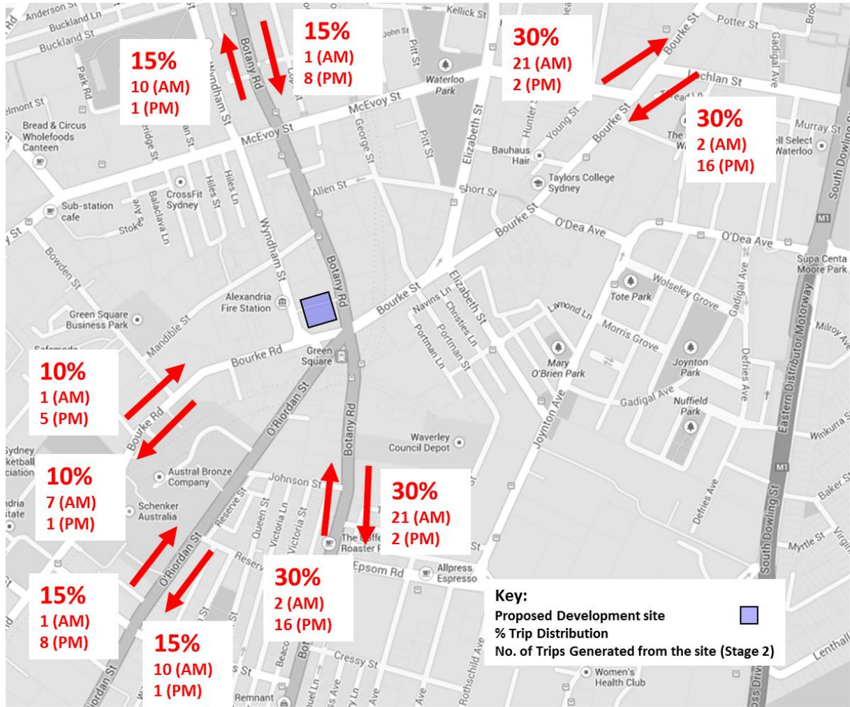
Figure 4 Trip Generation and Distribution for AM and PM Peak Hour (Stage 2 development)
