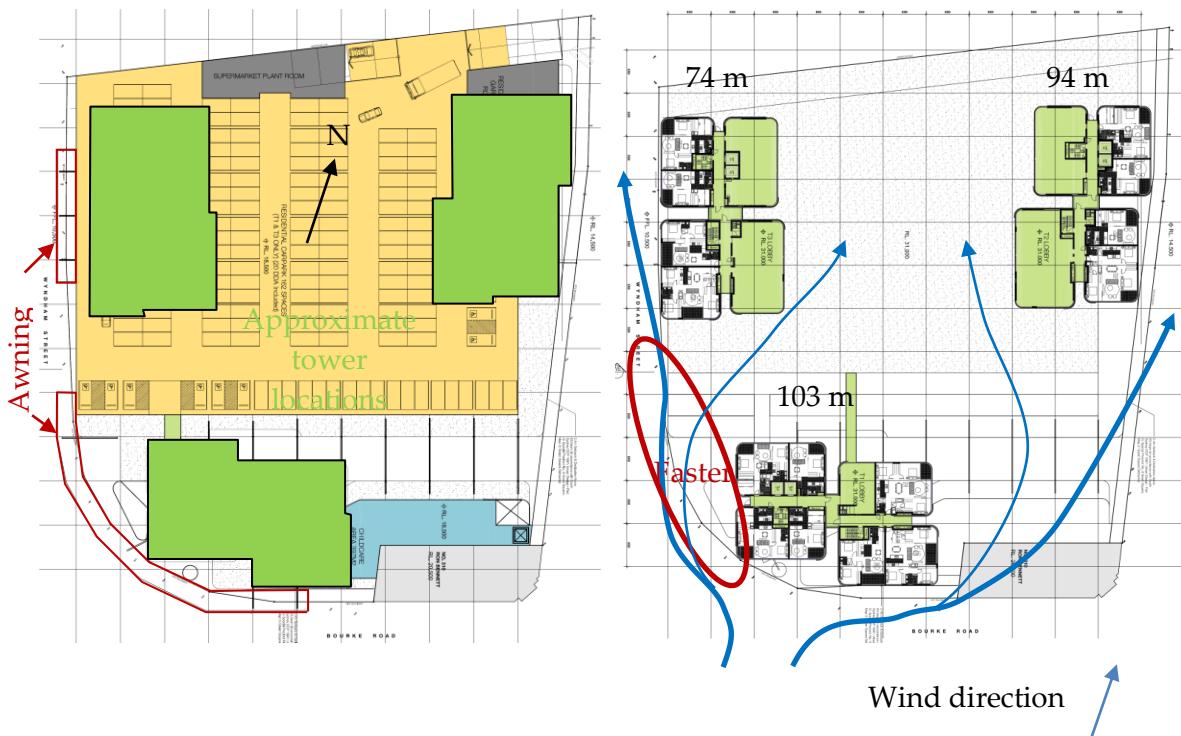
Figure 1: Plan view of the proposed development: revised (L), and previous showing wind flow patterns for winds from the south (R)
